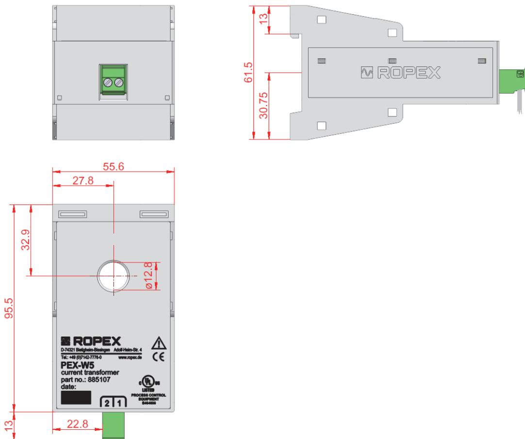
Mounting on DIN-rail 35 x 7.5 mm or 35 x 15 mm (DIN EN 50022).
