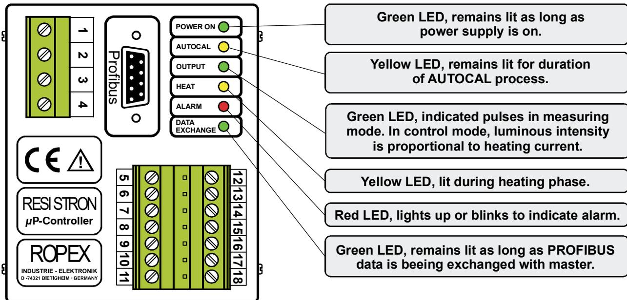
In addition to the functions shown in the diagram above, various controller operating states are indicated by the LEDs. These states are described in detail in the table below:
