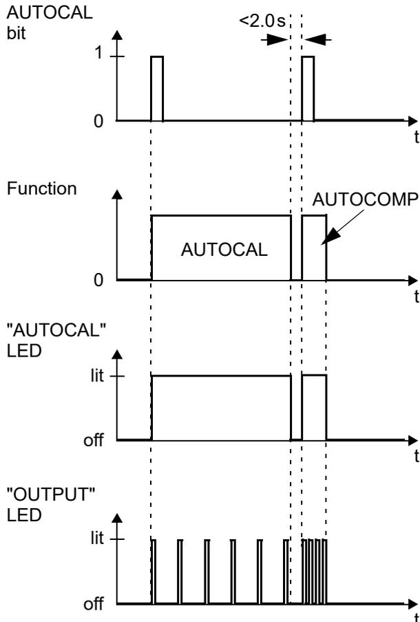
The "OUTPUT" LED blinks repeatedly when the "AUTOCOMP" function is executed and the actual value output (terminals 17+14) is set to 0...3°C (i.e. app. 0 VDC).
