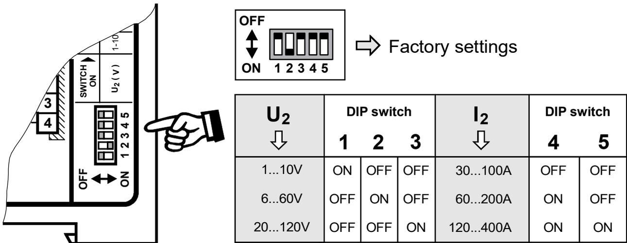
If the secondary current  $I_2$  is less than 30A, the secondary high-current wire must be laid twice (or several times) through the PEX-W3 or PEX-W4 current transformer (↪ ROPEX Application Report).
