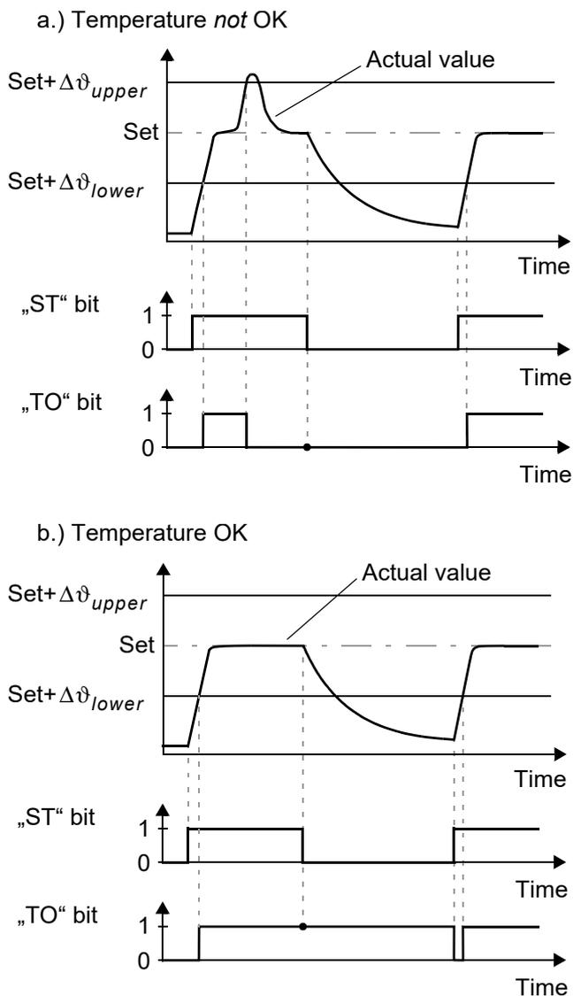
For controllers with software revision 100, 101 and 102 the configuration for the „TO“ bit can be set via the ROPEX visualization software. As of software revision 103 the configuration for the „TO“ bit is set in the PROFIBUS parameter data (or the DPV1 protocol extension). A configuration with the ROPEX visualization software is no more possible.
