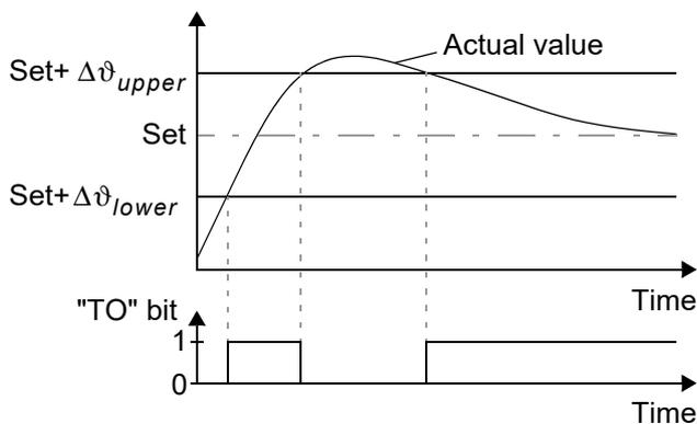
Unlike the "Temperature reached" status bit ("TE" bit), the actual temperature is evaluated independently of the control mode.
