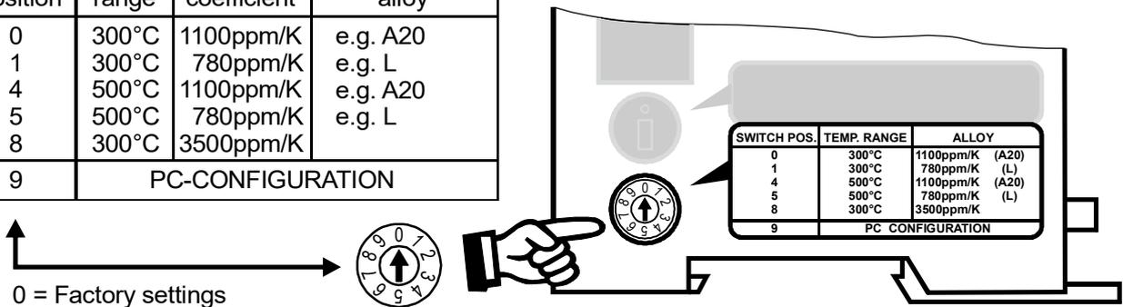
The settings for a temperature coefficient of 780ppm (switch position 1 and 5) are only available on controllers manufactured as of October 2003.
