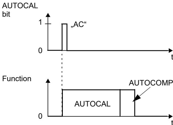
The "OUTPUT" LED blinks repeatedly when the "AUTOCOMP" function is executed and the actual value output (terminals 17+14) is set to 0...3°C (i.e. app. 0 VDC).
