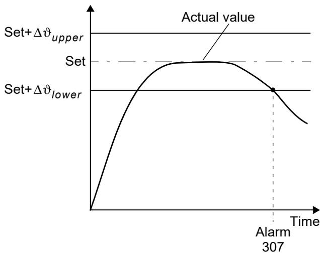
If the temperature diagnosis is not activated by the time the "START" bit is deactivated (i.e. if the ACTUAL temperature does not exceed the upper or lower tolerance band limit), the corresponding error code (309, 310) is indicated and the alarm relay is switched.
