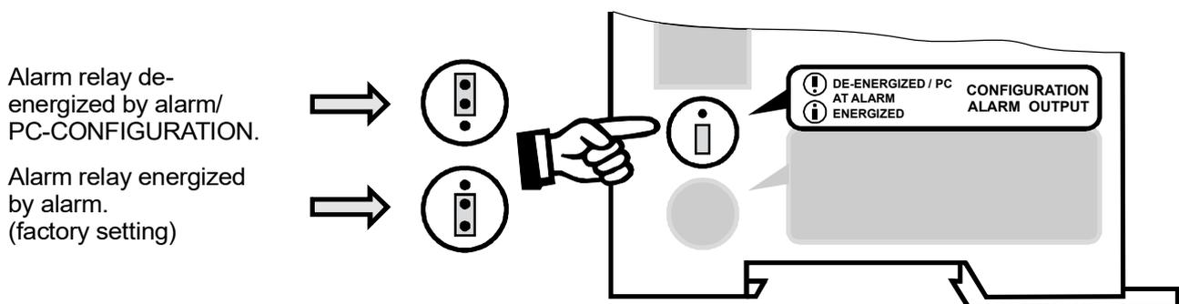
**!** If the jumper is not inserted, the alarm relay is permanently energized when using a controller up to production date January 2006. The other functions of the controller (e.g. heating, AUTOCAL etc.) are not impaired by this.
