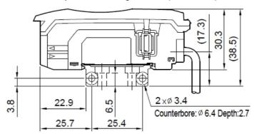
Bottom surface of amplifier mounting bracket
