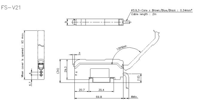
When mounting blacket is attached (Included in FS-V21)
