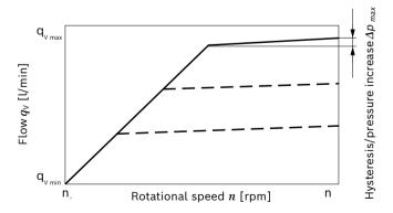
Characteristic curves valid at  $n_1$  = 1500 rpm and  $t_{fluid}$  = 50 °C.
