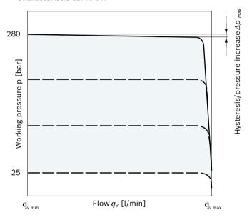
Characteristic curve valid for  $n_1$  = 1500 rpm and  $t_{fluid}$  = 50 °C.
