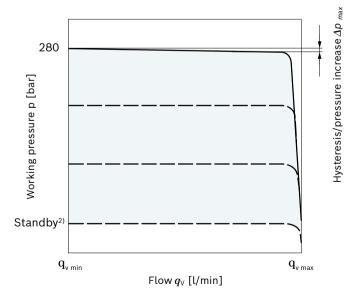
Characteristic curve valid for  $n_1$  = 1500 rpm and  $t_{fluid}$  = 50 °C.
