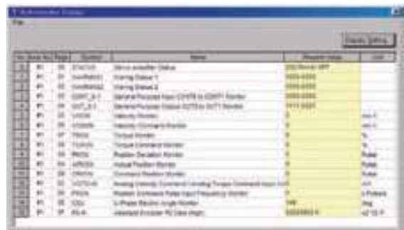
Multi-monitor Display: Simultaneous monitoring of operational status of multiple servo amplifiers networked to a PC.
