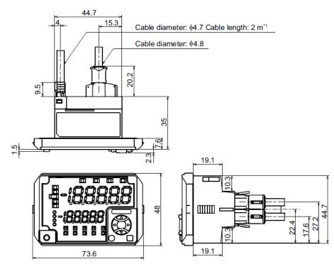
\*1 Cable specification : IG-1500 12 cores, Nominal cross-section area brown/blue: 0.20 mm<sup>2</sup>, others 0.15 mm<sup>2</sup> : IG-1550 8 cores, Nominal cross-section area: 0.15 mm<sup>2</sup>
